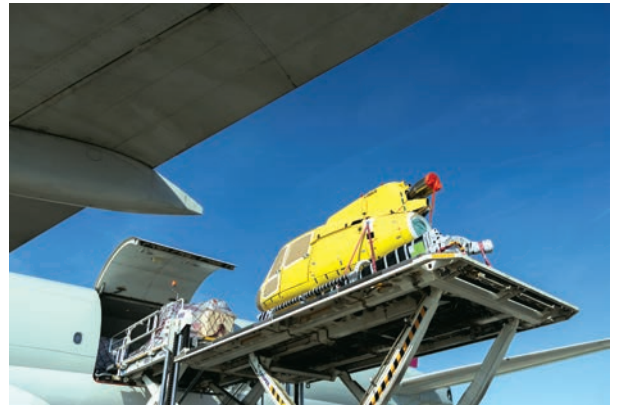
Specialised cargo handling: Loading a disassembled helicopter fuselage at Charles de Gaulle Airport.
